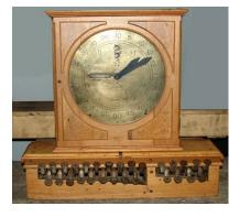
The first cash register was invented by James Ritty in 1883. Ritty was a saloon keeper in Ohio and nicknamed the invention the "incorruptible cashier." The machine used metal taps and simple mechanics to record sales. A bell sounded when a sale was completed, leading to the phrase "ringing up" — which we still use today.
